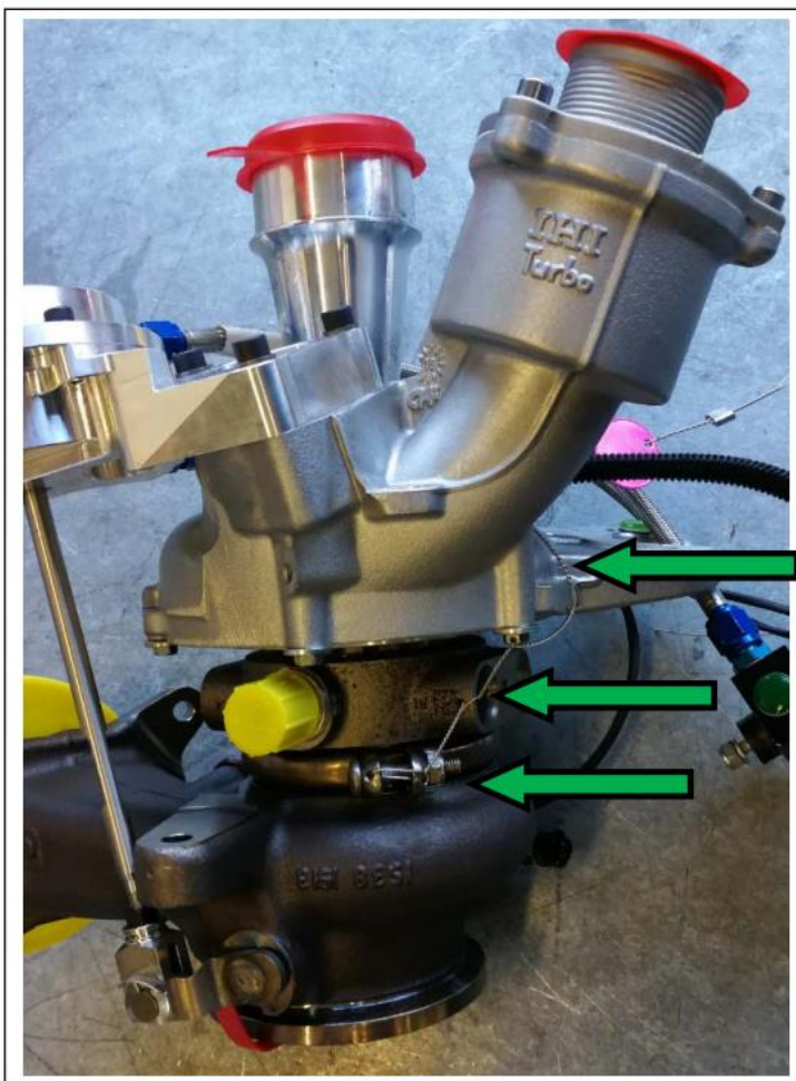
Example how to route wire through housing and exhaust (base part + mounting bolt)
